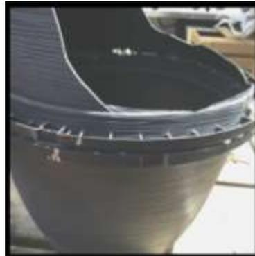
\*Tie-wraps were used to hold the two parts together while the glue dried.
